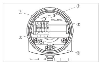
Electronics and connection compartment - transistor output
