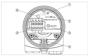
Electronics and connection compartment - NAMUR output
