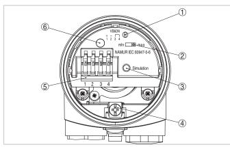
Electronics and connection compartment - NAMUR output
