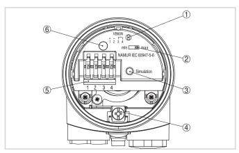
Electronics and connection compartment - NAMUR output
