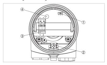
Electronics module - Two-wire output
