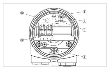
Oscillator - Transistor output
