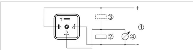
Wiring plan - Three-wire 1 x transistor or 4 ... 20 mA
